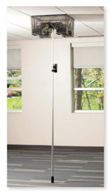
Once the hood is placed correctly, twist the pole to adjust the pole length so that it reaches the floor supporting the hood itself. If the hood is not securely in place, then re-adjust the pole length.
